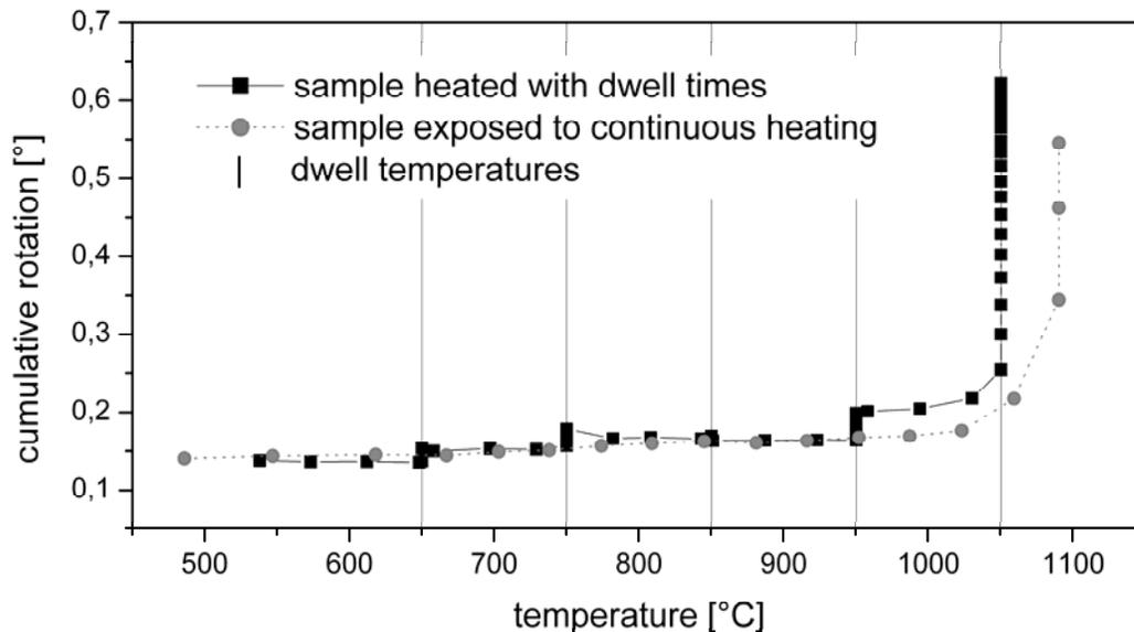
Figure 2: Differential and cumulative rotation vs. temperature. Monocrystalline spherical copper particles with radii of  $30\mu\text{m}$ . Heating rate: 10K/min. Dwell time 60min for each temperature.
