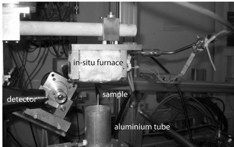
Figure 1: Tomography setup including the in-situ furnace. Here, the furnace has been lifted to change the sample.
