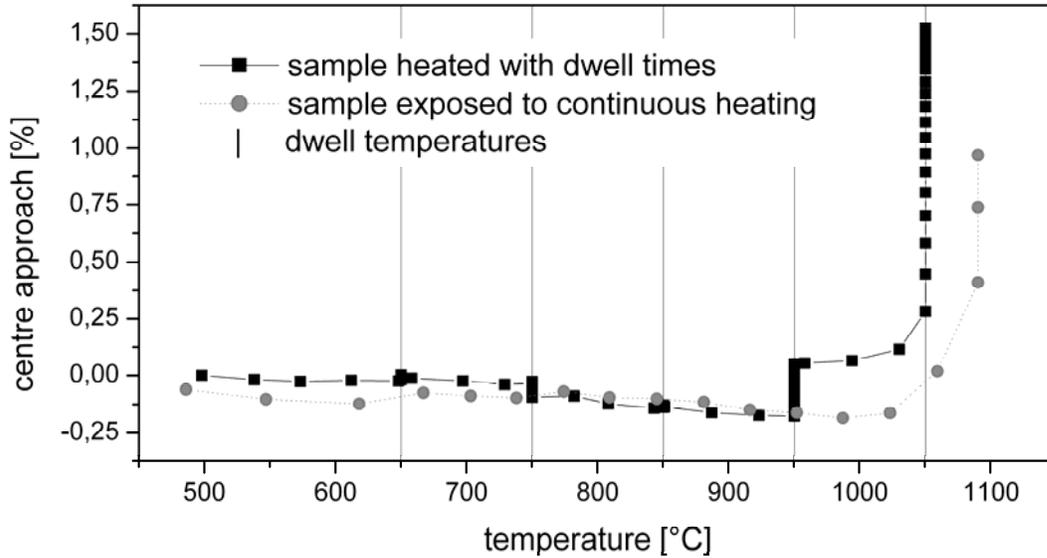
Figure 3: Centre approach vs. temperature. Monocrystalline spherical copper particles with radii of 30 $\mu$ m. Heating rate: 10K/min. Dwell time 60min for each temperature.
