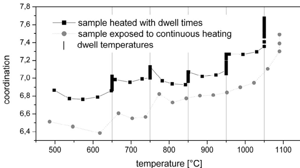
Figure 4: Number of contact partners vs. temperature. Monocrystalline spherical copper particles with radii of 30 $\mu$ m. Heating rate: 10K/min. Dwell time 60min each.
