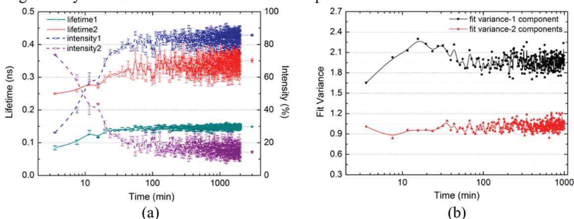
Figure 1. (a) Decomposition of two lifetime components in Al-0.005%Si alloy by applying the “low statistics method”. For comparison, the components obtained from “high statistics method” are also shown as solid symbols. (b) Variances of one and two lifetime components fits, where the results of the latter are shown in (a).
