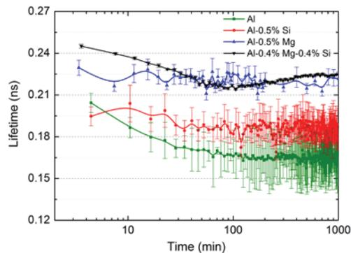
Figure 4. Average positron lifetime evolution during NA. For Al-0.4%Mg-0.4%Si, the spectrum was processed with single component fitting. For pure Al, Al-0.5%Mg and Al-0.5%Si alloys, 2 components were fitted.
