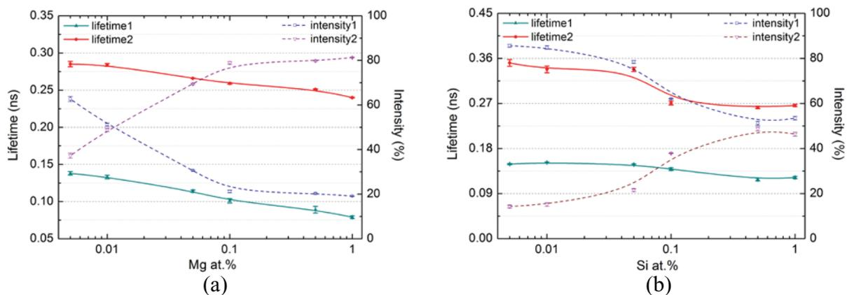
Figure 3. Dependence of positron lifetimes and intensities after 3000 min of NA on solute concentration in (a) Al-Mg alloys and (b) Al-Si alloys. Spline interpolations serve as guiding lines.
