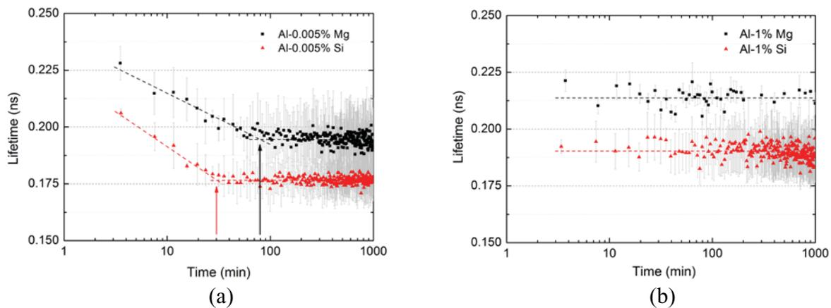
Figure 2. Evolution of the average lifetime during NA in alloys containing (a) 0.005% Mg/Si and (b) 1% Mg/Si. Arrows indicate the NA time when lifetimes reach to stable values.
