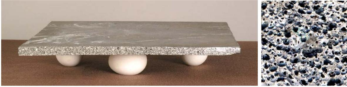
**Figure 6.** Aluminium alloy foam made by applying the Alcoa process involving  $\text{CaCO}_3$  as a blowing agent. a) entire foam panel, b) microstructure (Courtesy Dan Bryant).
