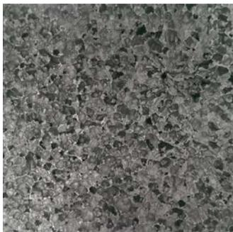
**Figure 5.** Typical morphology of an 'Alporas' foam. Picture taken from a sample handout by Shinko Wire. Co. Width of field 90 mm.
