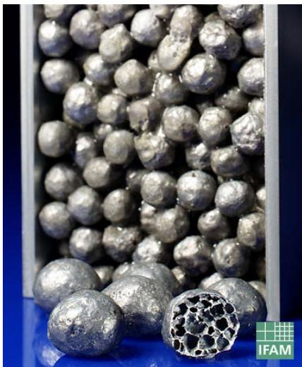
**Figure 10.** Composite structure comprising aluminium foam spheres that have been bonded together to form a filling of a tube. Courtesy Fraunhofer IFAM, Bremen.
