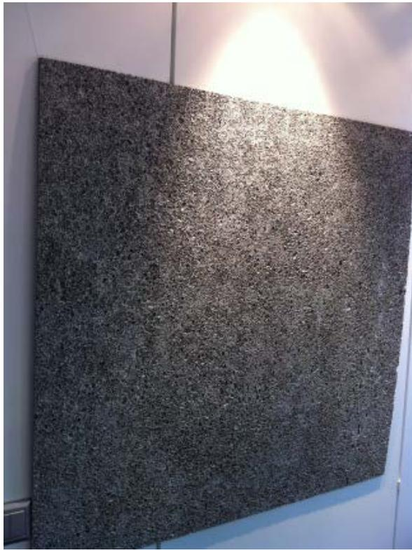
Figure 4. 1×1 m<sup>2</sup> large AFS sliced in the panel plane.
