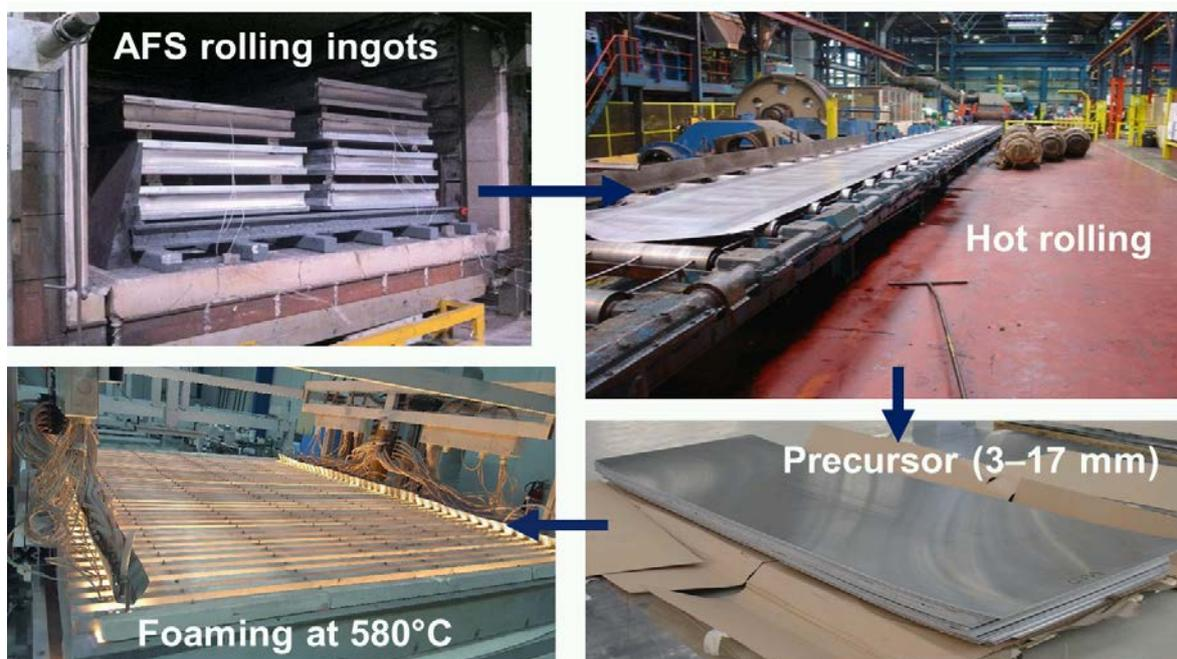
**Figure 2.** Images taken from various stages of AFS precursor manufacture. Upper left: Powder-filled ingots read for rolling, right: rolling process, lower right: rolled three-layer composites after rolling and cutting, lower left: foaming furnace.
