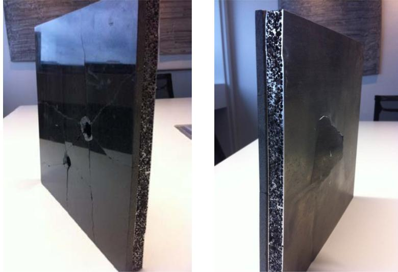
Figure 8. Composite of an AFS panel with a polished granite front plate hit by a bullet. The AFS had 1.8 mm face sheets and a 20 mm foam core, while the granite plate was 8 mm thick.
