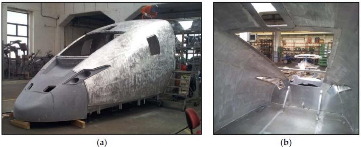
Figure 7. (a) Prototype of German high velocity train ICE made of welded aluminium foam sandwich. (b) view of the interior demonstrating the low number of components required (courtesy of Thomas Hipke, IWU, Chemnitz, Germany and Voith Engineering, Chemnitz, Germany).
