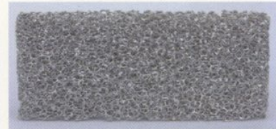
Aluminium foam (photo: METALL)
