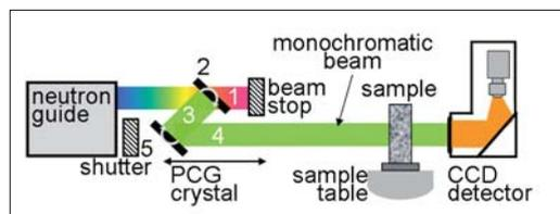
**Fig. 1:** Schematic sketch of CONRAD including the double monochromator device: (1) upper guide and neutron beam (2) first PG(002) monochromator, (3) diffracted monochromatic neutron beam, (4) second PG(002) monochromator, (5) lower guide and shutter of lower part of the neutron beam
