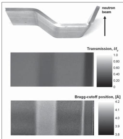
**Fig. 4:** Steel plate ( $50 \times 10 \text{ mm}^2$ ) of 5 mm thickness was deformed – photo on the top. The radiography image is shown in the middle. 2D mapped position of the Bragg edge for each pixel in the deformed plate is shown in the bottom image. The obtained map can be related to the residual stress distribution in the plate.
