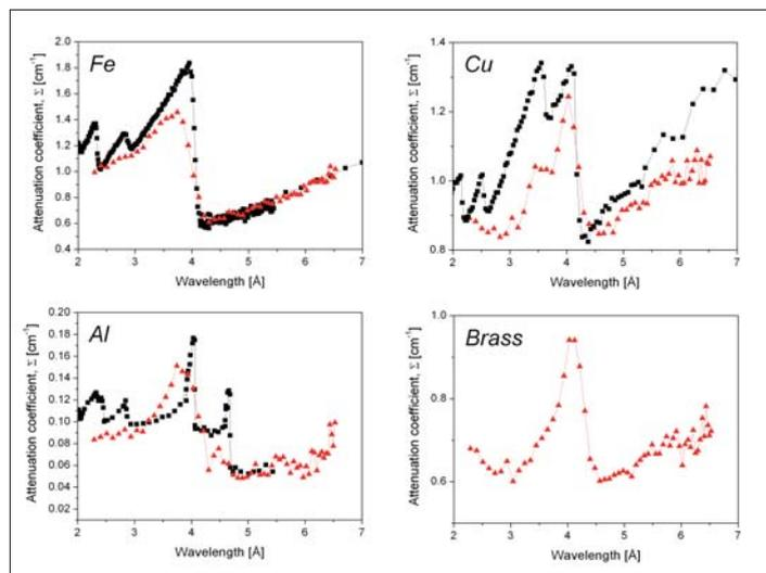
**Fig. 2(a) – (d):** Tabulated (dark) and radiographically (light) measured attenuation coefficients of Al, Fe, Brass and Copper. The measured values are smeared due to the rather large mosaic spread of the C- crystals.
