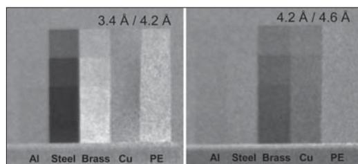
**Fig. 3:** Quotient images at wavelengths where the attenuation coefficients for Cu (left) and Fe (right) stay without change.
