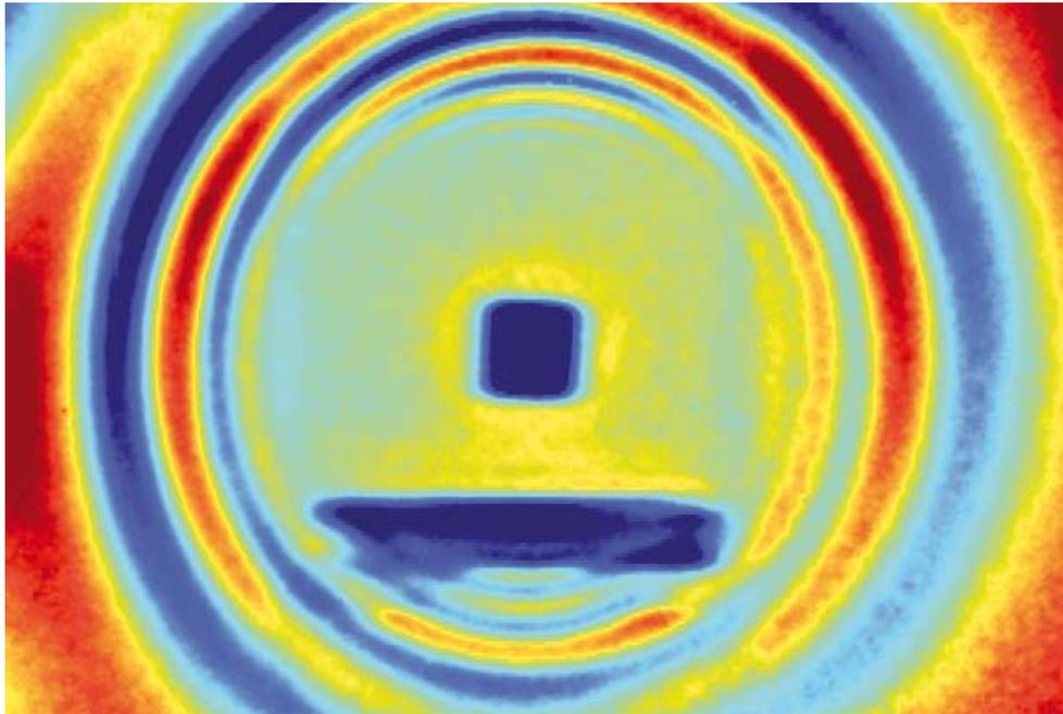
Figure 3: A radiograph showing the field lines around a bar magnet levitating over an yttrium barium copper oxide (YBCO) superconductor, a result of the so called Meissner effect. In its superconducting state the YBCO expels all magnetic fields and thus repels the permanent magnet.
