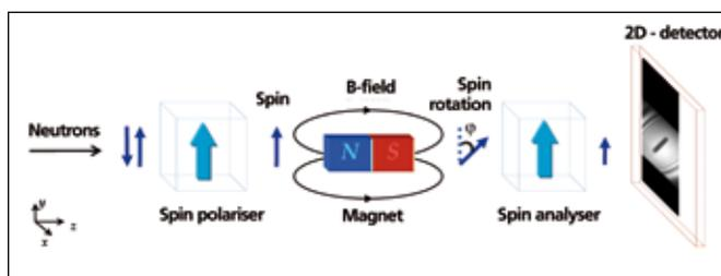
Figure 1: Schematic diagram of the set up used for imaging magnetic materials on CONRAD. The neutron beam is polarized, allowed to precess around a magnetic field, analysed, and then detected. Note how the intensity (dark blue arrow) behind the analyser is smaller than the intensity behind the polarizer.
