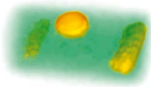
Figure 4: A three dimensional reconstruction of trapped flux (yellow regions left and right) inside a polycrystalline cylinder of lead. When cooled to below its critical temperature in the presence of a weak magnetic field some flux is present inside due to defects and grain boundaries, and this remains trapped even after the field is switched off.
