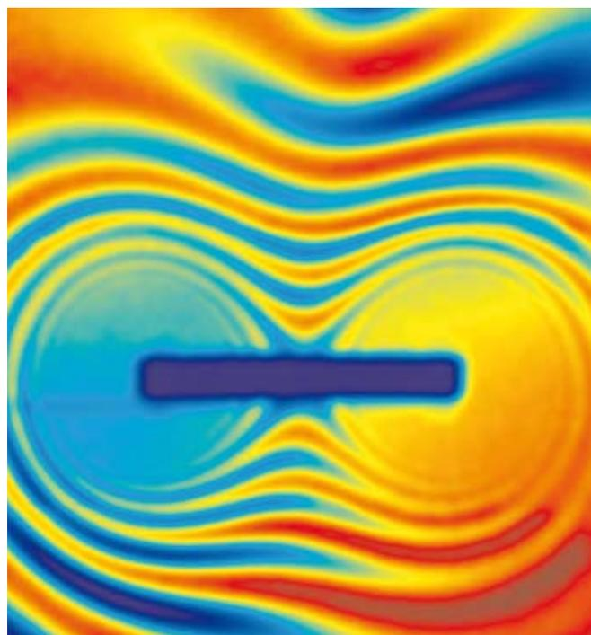
Figure 2: A radiograph showing the field lines surrounding a bar magnet. The magnetic field decreases in strength with distance from the magnet, resulting in a series of maxima and minima, where the beam polarization is sequentially parallel or anti-parallel, respectively, to the analyser. Very close to the magnets (where the field is strongest), the field lines are too close together to be resolved spatially.
