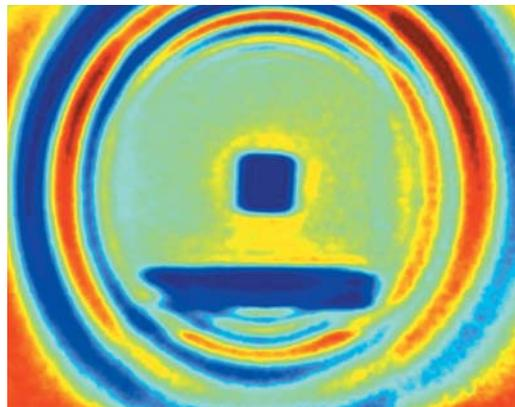
Fig. 3 — A radiograph showing the field lines around a bar magnet levitating over an yttrium-barium-copper-oxide (YBCO) superconductor, a result of the so-called Meissner effect. In its superconducting state, the YBCO expels all magnetic fields and thus repels the permanent magnet.
