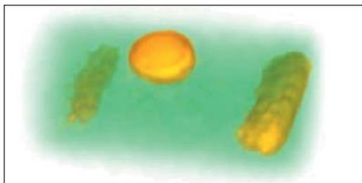
Fig. 4 — A three-dimensional reconstruction of trapped flux (yellow regions left and right) inside a polycrystalline cylinder of lead. When cooled to below its critical temperature in the presence of a weak magnetic field, some flux is present inside due to defects and grain boundaries, and this remains trapped even after the field is switched off.
