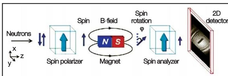
Fig. 1 — Schematic diagram of the setup for imaging magnetic materials on CONRAD. The neutron beam is polarized, allowed to precess around a magnetic field, analyzed, and then detected. Note how the intensity (dark blue arrow) behind the analyzer is smaller than the intensity behind the polarizer.
