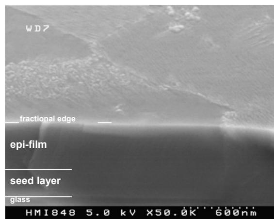
**Figure 2:** Fractional edge and surface of a 400 nm thick crystalline Si film grown on a poly-Si seed layer on glass (SEM image).
