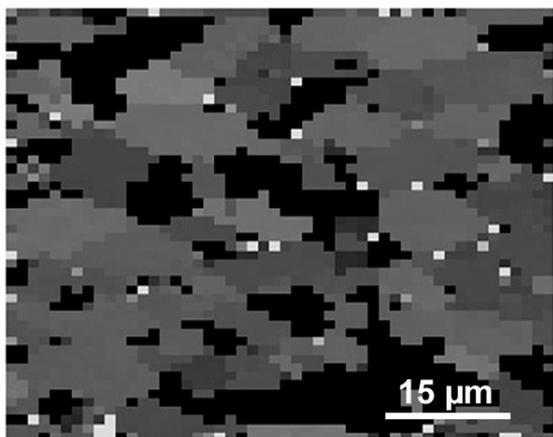
**Figure 3:** EBSD orientation map of the Si film shown in Fig. 2 (gray regions: epitaxially thickened grains, black regions: finecrystalline thickened grains).
