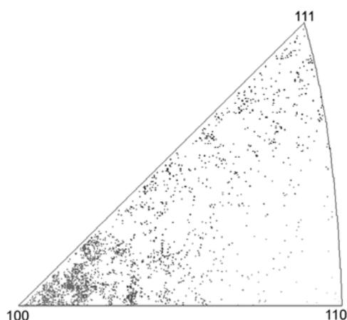
**Figure 1:** EBSD pole figure of a poly-Si seed layer on glass made by ALILE showing the statistics of grain orientation.
