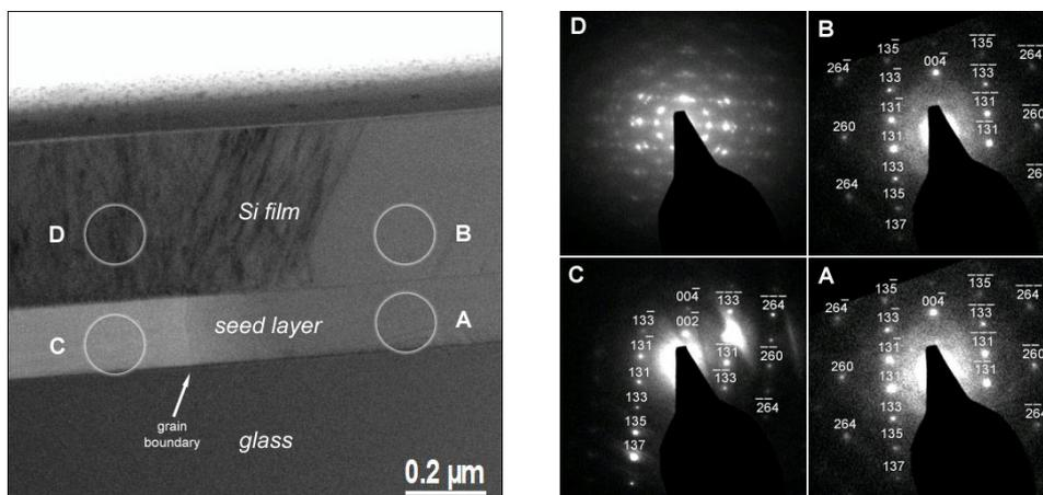
**Figure 4:** TEM cross section (left) and diffraction pattern (right) of the poly-Si film deposited on a seed layer on glass. The circles mark the positions of the selected area aperture for electron diffraction. The diffraction images are aligned with respect to the neighbouring TEM image.
