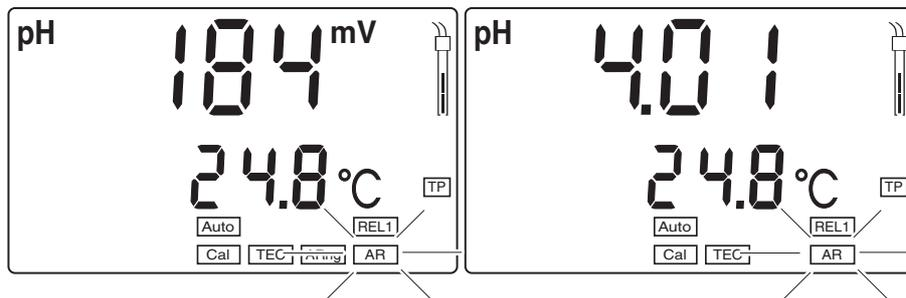
10 | When the measured value is stable, *AR* disappears. The value of the slope (mV/pH) appears on the display. The sensor symbol shows the evaluation of the current calibration.
