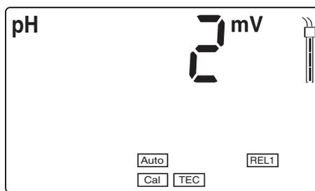
12 | Switch to the measuring mode with **<M>**.
