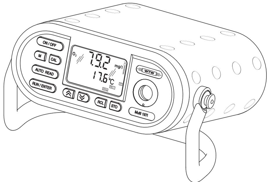
**Portable pH / oxygen / conductivity measuring instrument**
