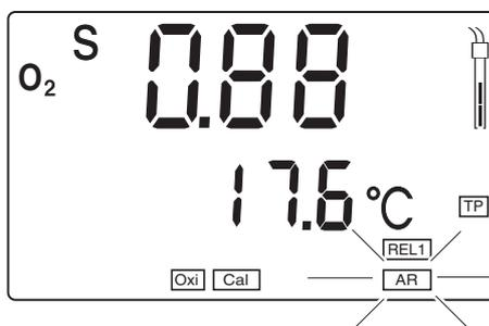
6 As soon as a stable value is achieved the AR display stops flashing. The calibration is finished then. The value of the relative slope appears on the display. The sensor symbol shows the sensor evaluation (see page 33).
