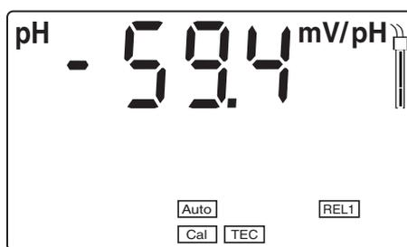
11 | Press the **<RUN/ENTER>** key. The value of the asymmetry (mV) appears on the display.
