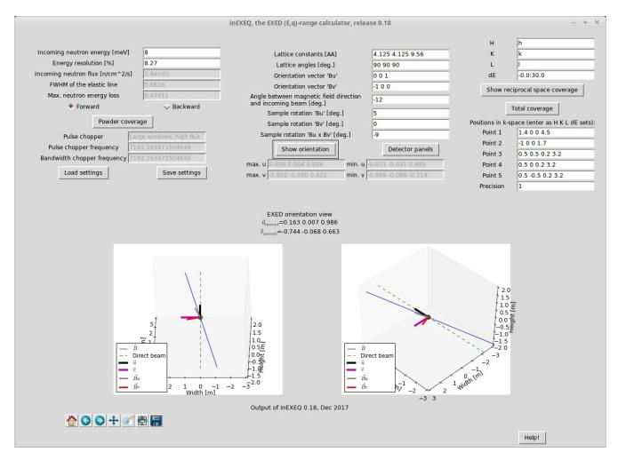
Here the direction of the **Bu** and **Bv** vectors is shown in real space, relative to the neutron beam and magnetic field directions.
