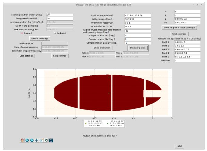
Detector view shows the real-space view of the detector panels. The shadow of the magnet cone, beamstop and the gaps between the panels are included in the plot.
