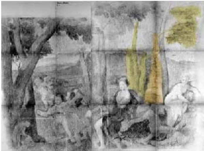
Fig. 2: Nicolas Poussin, "Armida abducts the sleeping Rinaldo", 1st neutron autoradiography assembled from 12 image plate records: in order to investigate the whole picture, two separated irradiations were carried out and finally recomposed.
