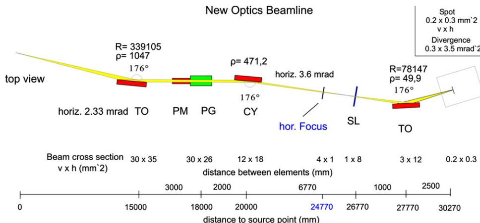
Fig. 1. Schematic layout of the new optics beamline at BESSY-II Dipol 1.1.
