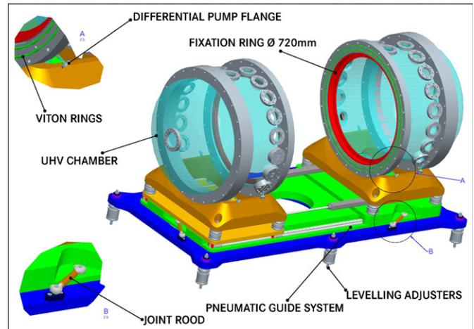
Fig. 8. The UHV-chamber for the reflectometer with the adjustable stand.
