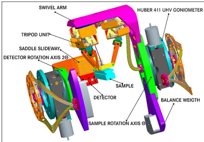
Fig. 6. Sample and detector rotation.
