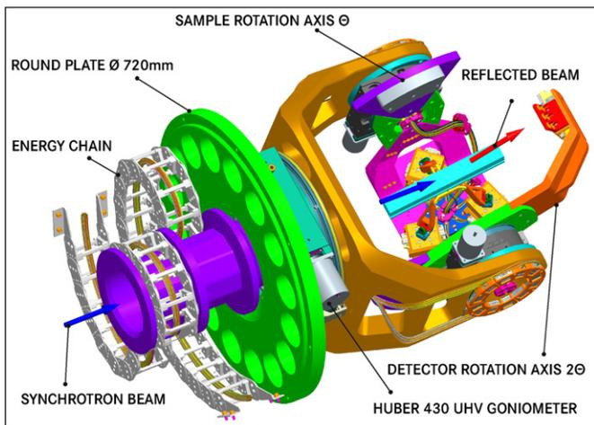
Fig. 7. Sample azimuthal rotation.
