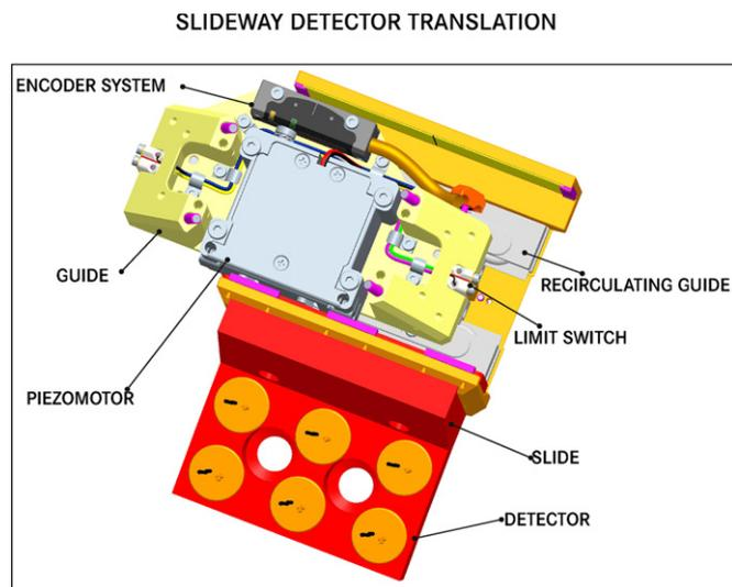
Fig. 5. The detector arm translation stage.
