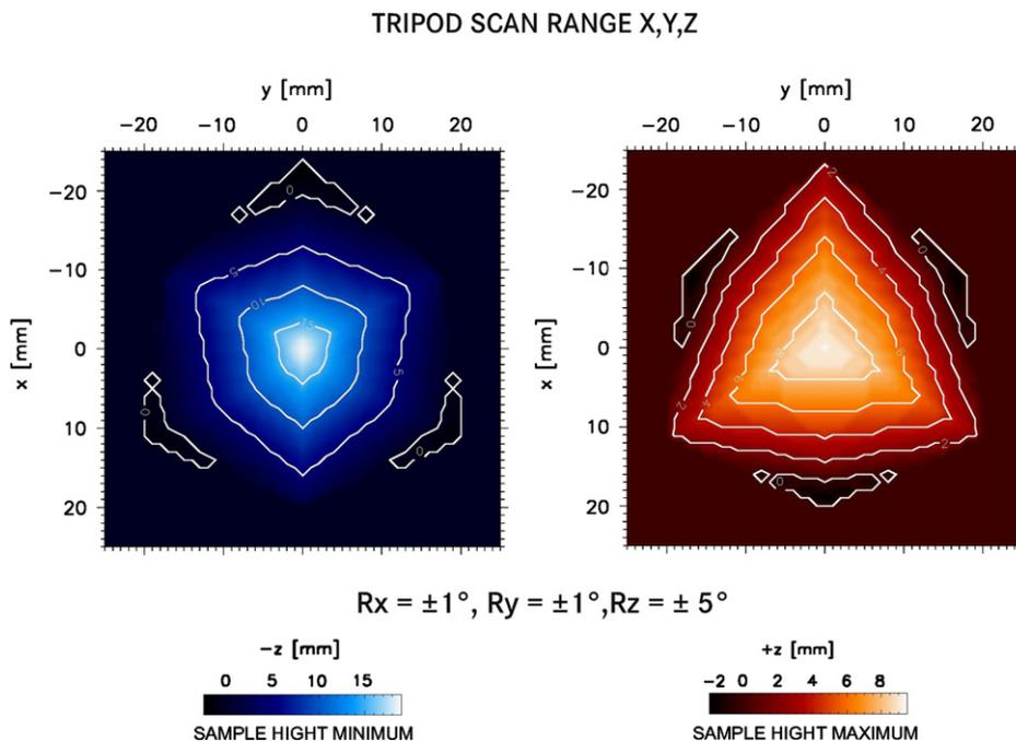
Fig. 4. The tripod unit scan range in the *x*- and *y*-directions as function of sample height for a fixed rotational range of *R<sub>x</sub>*, *R<sub>y</sub>* and *R<sub>z</sub>* as indicated.
