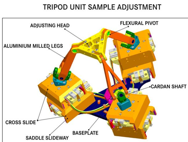
Fig. 3. The tripod unit for sample adjustment in six degrees of freedom.
