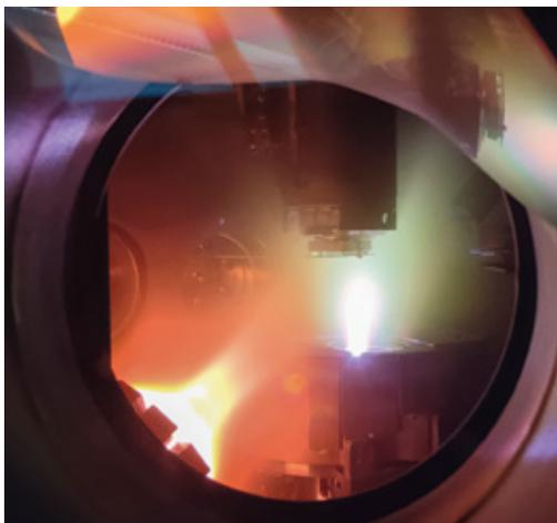
Pulsed laser deposition: An intense laser pulse hits a target containing the material, transforming it into a plasma which is then deposited as a thin film onto a substrate.
