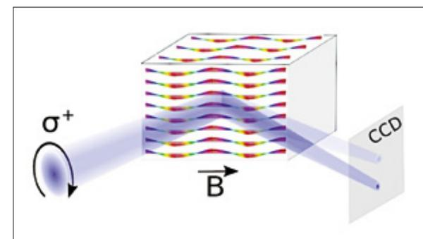
The picture reflects the main effect: A circular polarized soft-X-ray beam scatters off a crystal that exhibits a helical or conical magnetic order. This leads to two scattered beams of different intensity.
