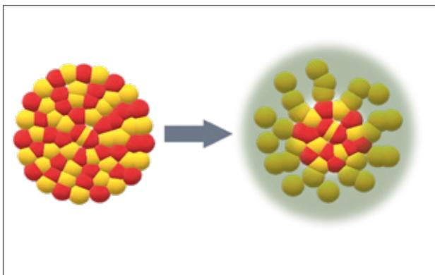
Crystalline nickel silicide (left) is chemically transformed into nanostructured material with excellent catalytic properties for the electrolytic splitting of water and the production of valuable nitrile compounds.
