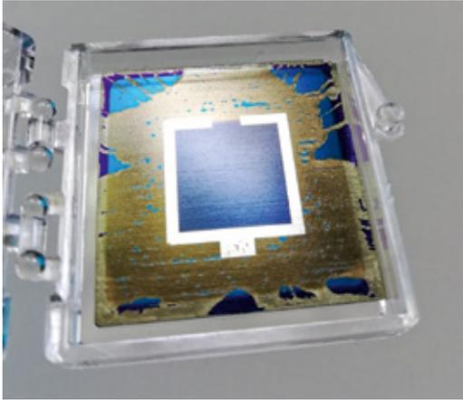
The HZB team has applied a perovskite top cell to a standard silicon cell. This tandem solar cell could achieve high efficiencies with further optimization.
