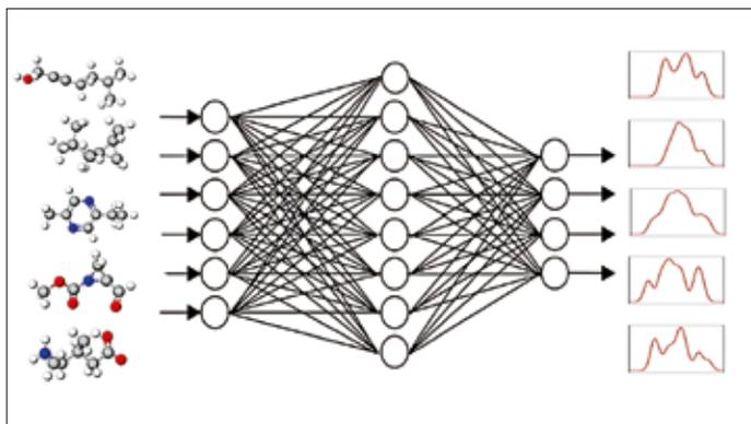
The graphical neural network GNN receives small molecules as input with the task of determining their spectral responses. By matching them with the known spectra, the GNN programme learns to calculate spectra reliably.
