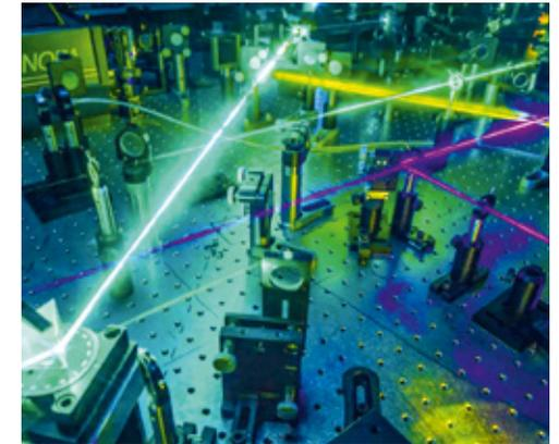
In the femtosecond laser laboratory, charge transport in semiconductors can be studied with terahertz and microwave spectroscopy. For this purpose, laser pulses first generate charge carriers in the material, which then absorb long-wave radiation (terahertz or microwaves) proportional to their mobility. © HZB
