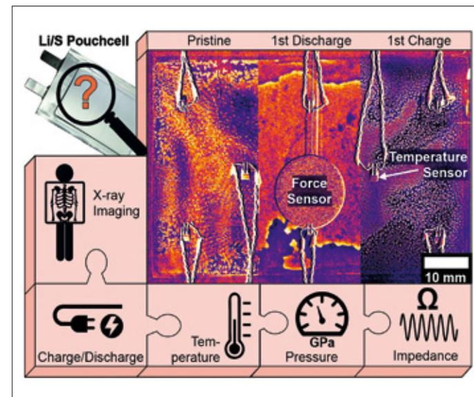
The radiographies of the cell before (left) and after the first discharge (centre) as well as after the first recharge (right). The accumulation of Sulphur-containing particles (bright spots) is visible. This combination of methods allows to compare pouch cells with different electrolytes and additives.
