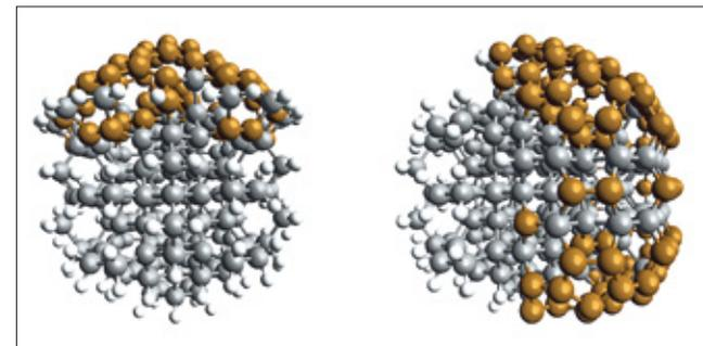
The illustration shows two variants of nanodiamond materials with different surfaces:  $\text{C}_{230}\text{H}_{106}$  on the left,  $\text{C}_{286}\text{H}_{68}$  on the right.  $\text{Sp}^3$  C atoms (diamond) black,  $\text{sp}^{3x}$  C atoms (fullerene-like) brown, H atoms: Light grey. © T. Kirschbaum/HZB
