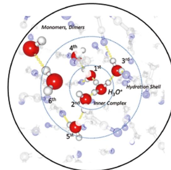
The spectral fingerprints of water molecules could be studied at BESSY II. The result: the electronic structure of the three innermost water molecules in an  $\text{H}_7\text{O}_3^+$  complex is drastically changed by the proton. In addition, the first hydrate shell of five other water molecules around this inner complex also changes, which the proton perceives via its long-range electric field.
