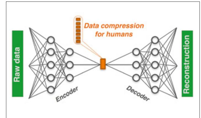
With the help of special neural networks, raw data can first be compressed and then reconstructed in such a way that it can be interpreted by scientists.
