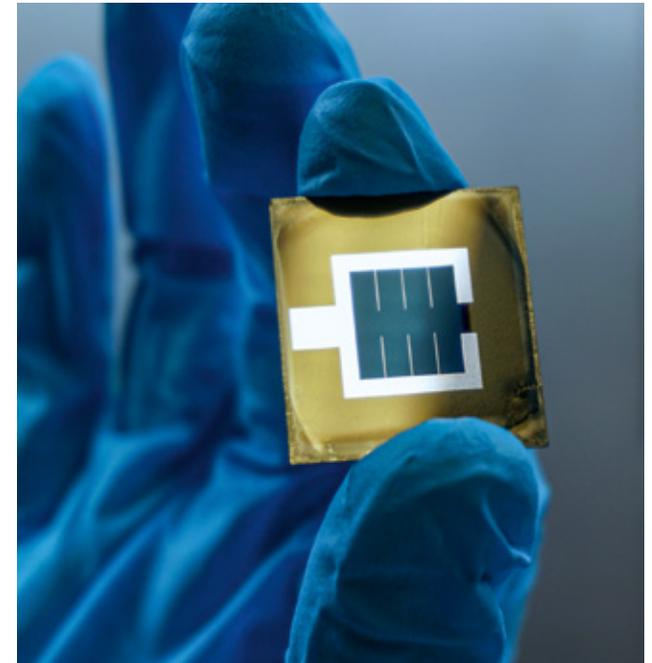
Photo of the perovskite/silicon tandem solar cell. You can see the active bluish area in the middle of the wafer, which is enclosed by the metallic, silvery electrode.
