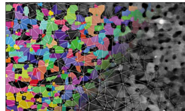
Electron microscope image of a silicon sample with nanocrystallites of different orientation (coloured), pores (black) and the pore network recognised by the image processing software (white grid lines).
