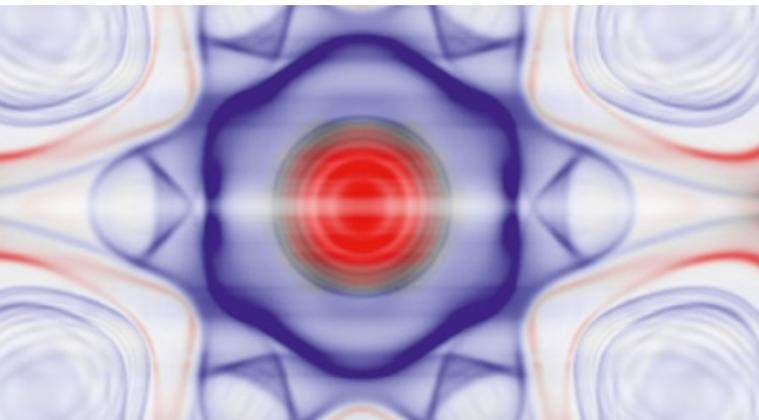
Using density functional theory and measurement data from spin-resolved photoemission, the team investigated the origin of the repeating Au(111) bands and resolved them as deep surface resonances. These resonances lead to an onion-like Fermi surface of Au(111). ©HZB
