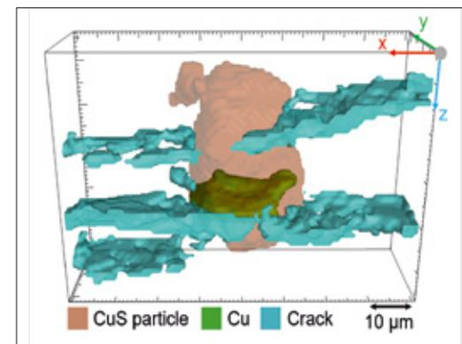
3D reconstruction of the formation of a copper crystallite in a copper sulfide particle (CuS) during the discharge of a lithium CuS solid-state battery. The volume expansion can lead to the formation of cracks (blue).
