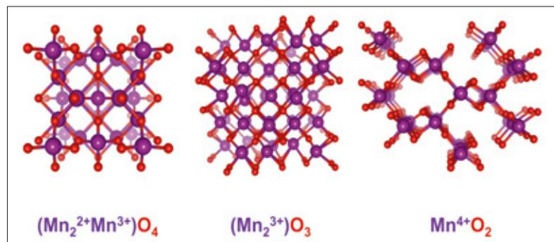
Manganese oxides come in many different structural variants. They are an exciting class of materials for electrocatalysts.
