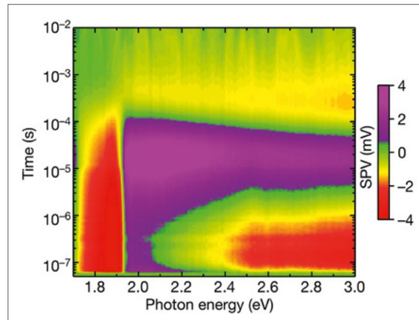
Contour plot of EH- $\text{Cu}_2\text{O}$ . The photovoltages are plotted as a function of photon energy (x-axis) and time (y-axis). Positive SPV signals (purple regions above 1.9 eV) correspond to the relaxation of holes trapped on {111} facets, whereas negative SPV signals (red regions) correspond to the relaxation of electrons trapped on {001} facets. © T. Dittrich/HZB
