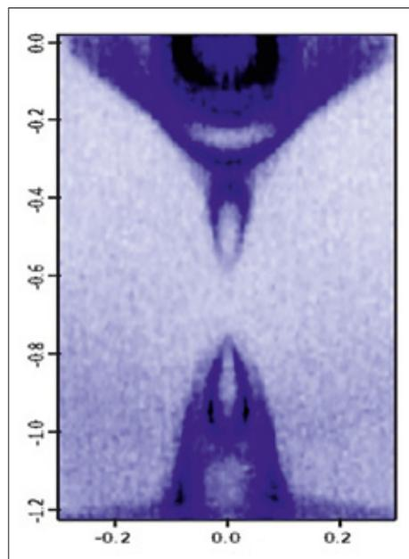
The experiment at the U125-2PGM undulator beamline of BESSY II shows bands with opposite curvature, so-called Fermi arcs.
