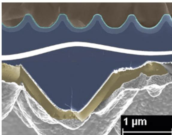
Scanning electron microscopy of perovskite silicon tandem cells in cross-section with nanotexture and back-reflector layer (golden). © P. Tockhorn/HZB
