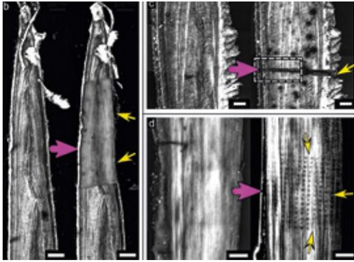
The images (b) show the collagen distribution in pike bones before (left) and after (right) a  $\mu$ CT experiment and (c) before (left) and after (right) an X-ray diffraction  $\mu$ CT experiment at the mySpot beamline, BESSY. Also (d) before (left) and after (right) a 2D mapping XRD mySpot experiment. The damaged areas appear dark marked with yellow arrows. Arrows in pink show the x-rays. © Charité Berlin/HZB
