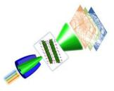
studied titanium dioxide rods illuminated by X-rays of various photon energies through a capillary condenser. A highresolution lens - not shown here - then forms an image of the objects. Source: HZB
