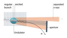
Schematic illustration of pulse picking by resonant excitation (PPRE): In regular operation the non-excited bunches (grey) emit undulator radiation on-axis. A
