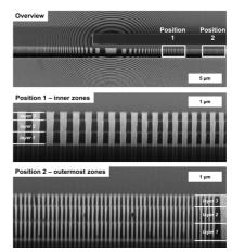
These scanning electron micrographs show how accurately the three Fresnel zone plates were positioned above one another. 3D X-ray optics of this kind allow the resolutions and optical intensities to be considerably improved.
