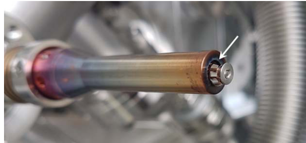
Figure 4. Copper cathode insert covered with a sputtered material (pointed with an arrow). The missing lip of the holding mechanism can be noted close to the arrow.
