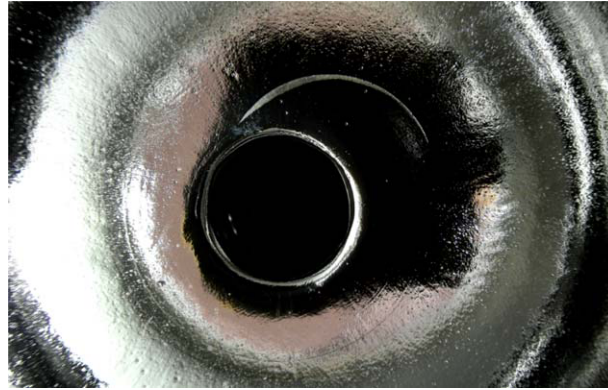
Figure 7. Optical image of Gun 1.1 back plate after collision with HPR nozzle. The dark area around the defect is a reflection of a camera.
