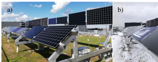
Fig. 1: Picture of the industrial module test setup in the roof laboratory in Berlin, Germany. All modules are MPP-tracked individually while rear side temperatures are measured as well as POA irradiance by monitoring cells. a) sunny day, b) after snow fall.
