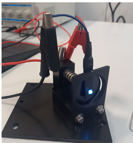
Figure 20. Photograph of the LED lamp fabricated with a UV chip (320 nm) under bias (4.4 V, 0.02 A) during the measurement.
