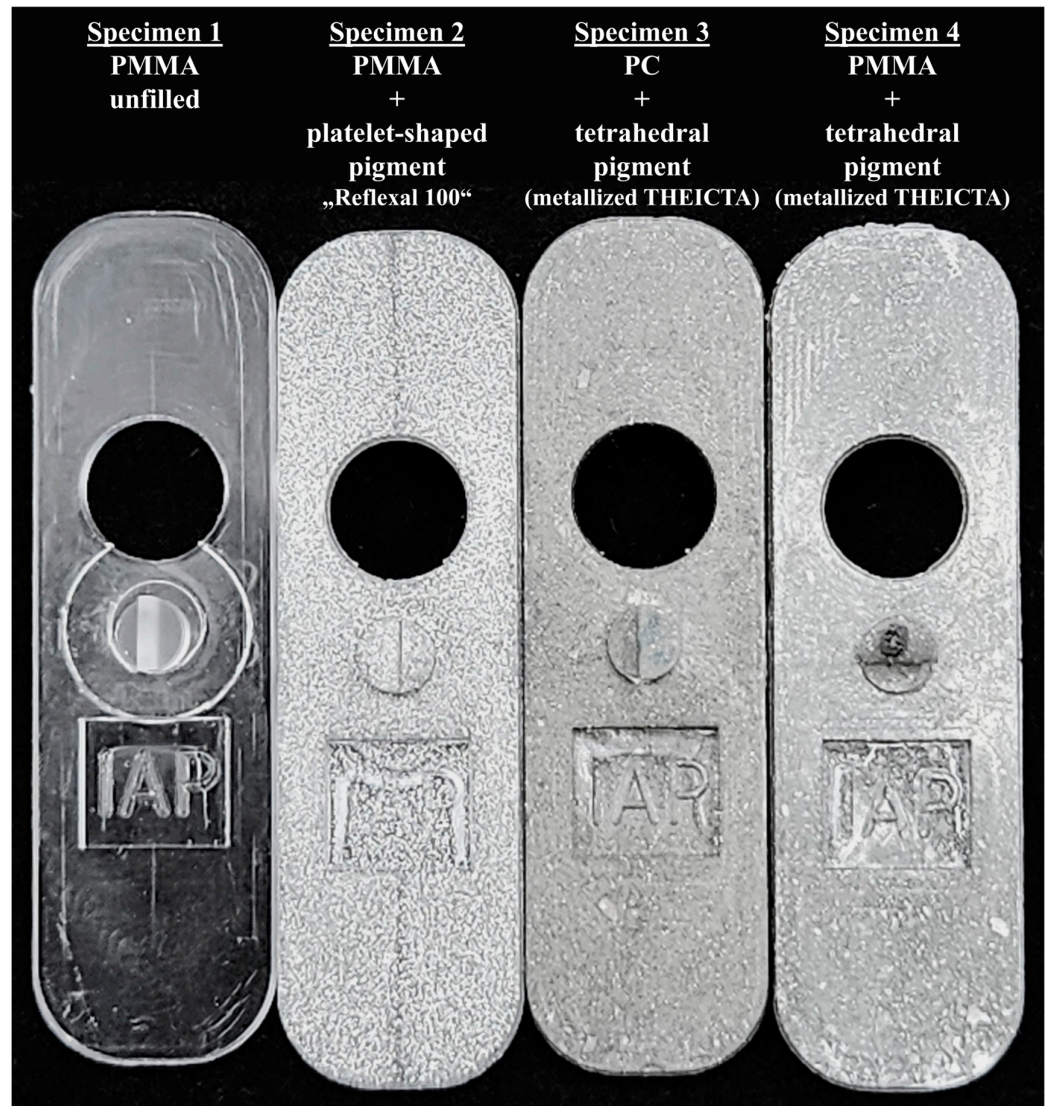
Figure 11. Injection-molded test specimens. The flowline prominent in the platelet-filled specimen is greatly reduced in the tetrahedron-filled specimen.
