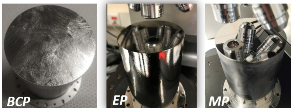
FIG. 2. The surface appearance of the QPR sample after various processing steps is shown from left to right: BCP, EP, and MP. In terms of quality, the BCP surface has low reflectivity, the EP surface shows moderate reflectivity, and the MP surface features a highly reflective, mirror-like finish. This variation in reflectivity results from differences in topography, as illustrated in Fig. 1.
