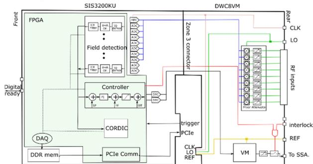
Figure 1: Diagram of the SIS8300KU (left) and DWC8VM (right) boards with single cavity firmware.
