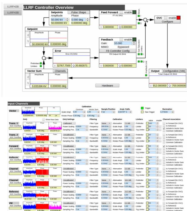
Figure 4: LLRF main control panel (up) and RF channels' panel (down).
