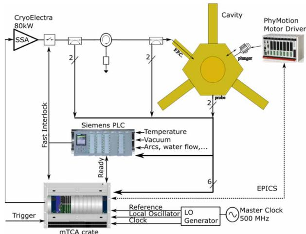
Figure 2: Complete setup composed by a mTCA crate, a Siemens PLC, a Cryoelectra SSA, a PhyMotion motor driver and a Local Oscillator Generator.
