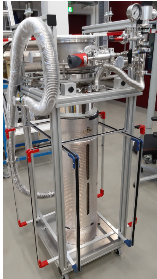
Figure 1: Picture of glass cryostat with two Helmholtz-coil pairs mounted to the aluminum frame creating field in x-direction (red corners) and y-direction (blue corners). Additionally, an insulated copper wire is wound around the cryostat's housing, forming a solenoid which creates field in z-direction.
