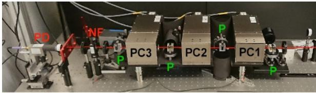
Figure 3: Signal detection setup at the undulator beamline: Three Pockels cells (PC) are placed between crossed polarizers (P). Additional filters (NF) can be placed in front of the photodiode (PD).
