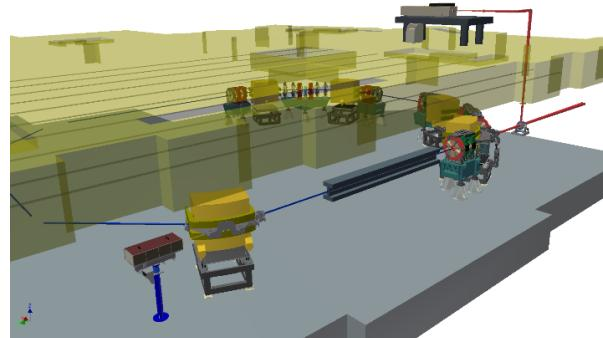
Figure 1: Schematics of the setup: The laser is operated inside the storage ring bunker and overlapped with the electron beam in the undulator straight section. The detection setup is placed in the MLS experimental hall.
