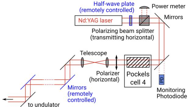
Figure 4: Setup inside the storage ring bunker: A Nd:YAG pulsed laser is used. The laser beam is blocked after the laser shot by a Pockels cell in order to prevent the seeding laser to enter the detection area.
