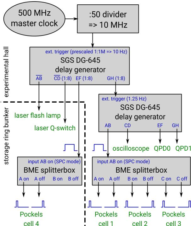
Figure 6: Trigger scheme of the experiment: the laser, the optical switches and the beam imaging systems (QPD0, QPD1) are synchronised to the revolution frequency of the bunches.
