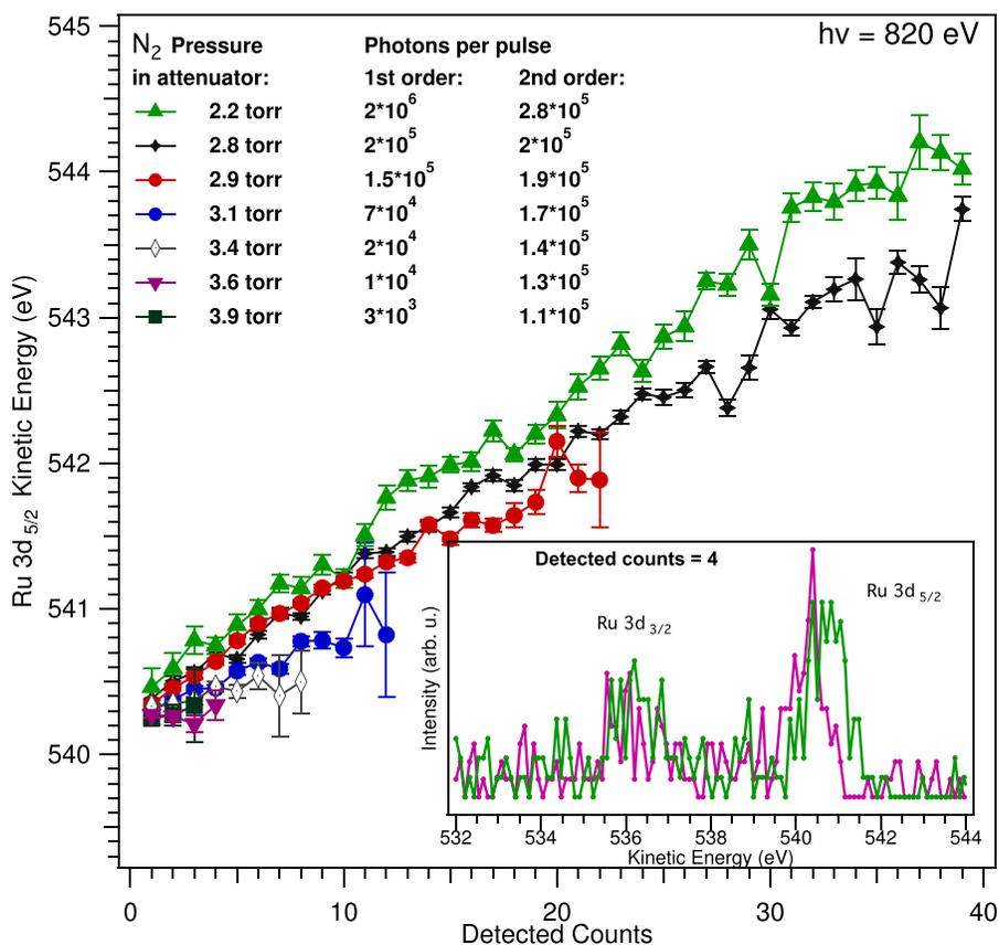
FIG. 2. Energy position of the Ru 3d<sub>5/2</sub> core level as a function of number of detected counts for different N<sub>2</sub> pressures in the gas attenuator. The estimated number of photons in first and second order is also reported. For each attenuation setting, the measurement lasted between 2 and 6 min. In the inset, the measured Ru 3d lines at two attenuations (colour encoded) with four detected counts in the analyzer are plotted.
