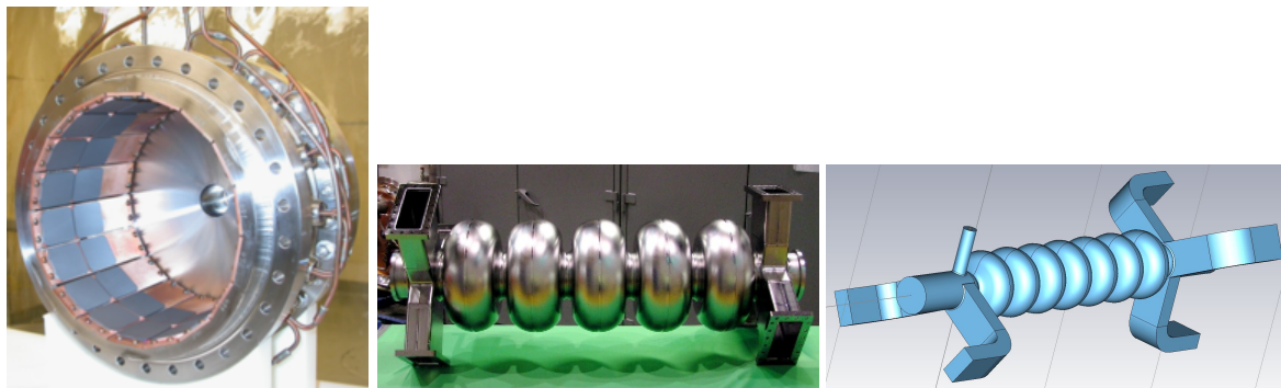
Figure 9: (left) Photograph of the Cornell electron storage ring beamline HOM load. Ferrite tiles (gray) are soldered to water-cooled elkonite plates that line the beam tube. HOMs that reach the load are quickly heavily damped by the ferrite. (middle) A prototype waveguide damped cavity developed by Jefferson Laboratory. (right) RF model used by HZB to simulate waveguide damping of an SRF cavity for BERLinPro.
