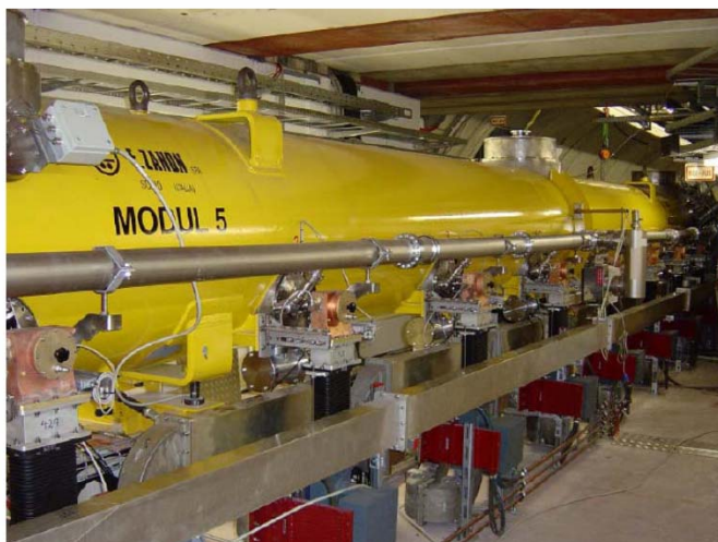
Figure 5.1: A TESLA cryo-module that will be the basis of both the STARS and BESSY FEL linacs.
