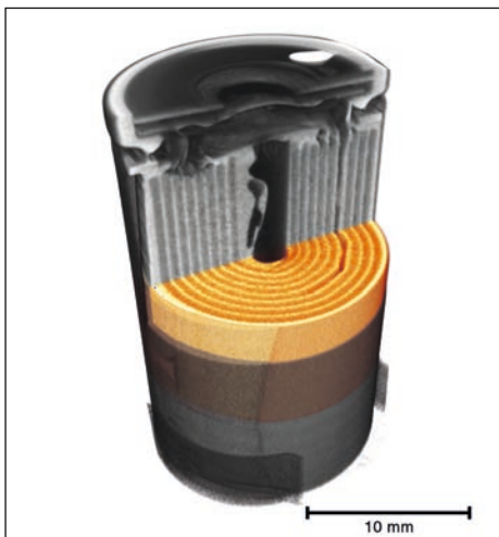
3-D view of a battery sliced open virtually. © T. Artt, I. Manke/HZB, R. Ziesche/UCL
