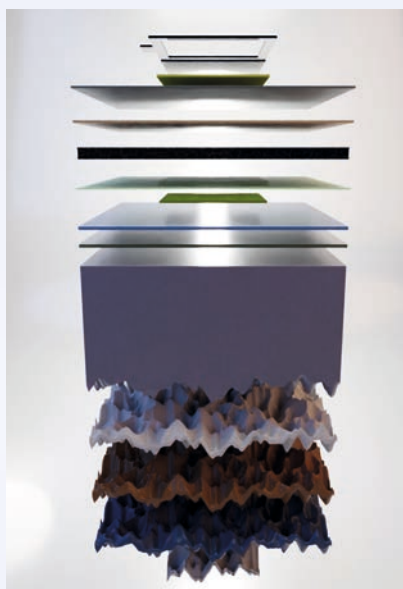
The illustration shows schematically the structure of the tandem solar cell. © HZB/ E. Köhnen
