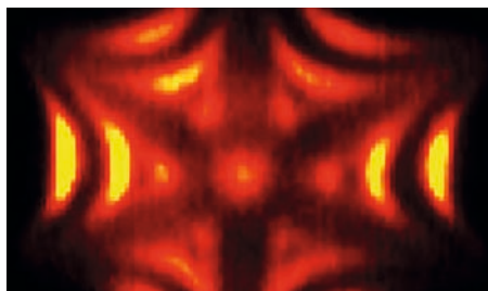
The Fermi surface of a GeTe Crystal (111) could be empirically determined at BESSY II. © HZB
