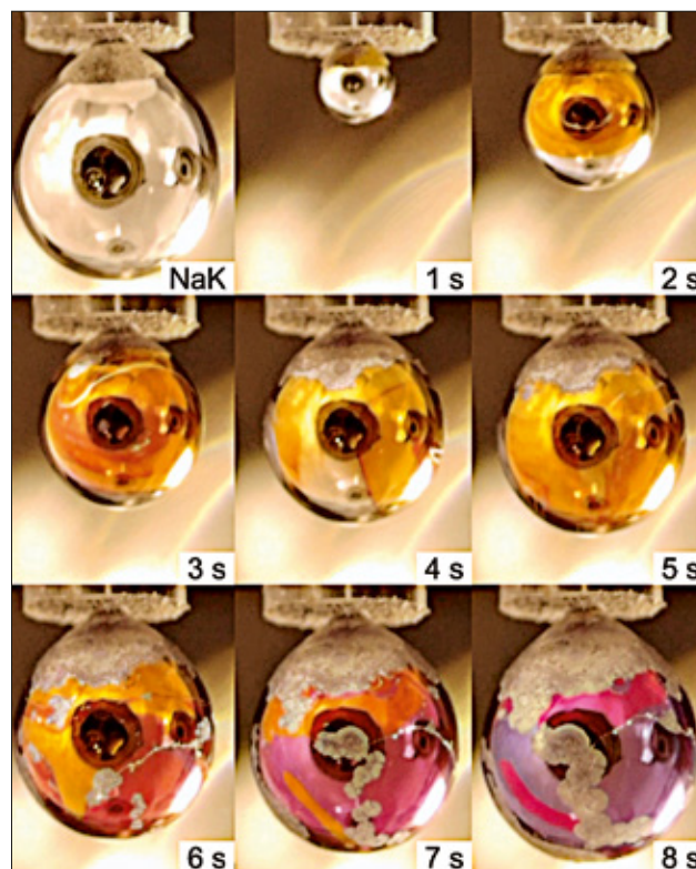
After about five seconds, a thin film of metallic water has formed around the sodium-potassium drop, recognisable by the golden shimmer. © HZB
