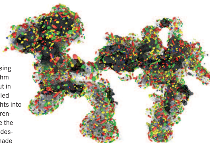
Catalyst nanoparticles (coloured) adhere to a substrate (grey), captured by electron tomography. Novel processing algorithms were used for this three-dimensional image.
