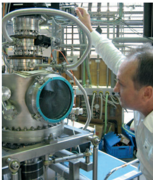
HZB scientist Florin Radu inspects a \text{BaTiO}_3 sample in the ALICE diffractometer.
