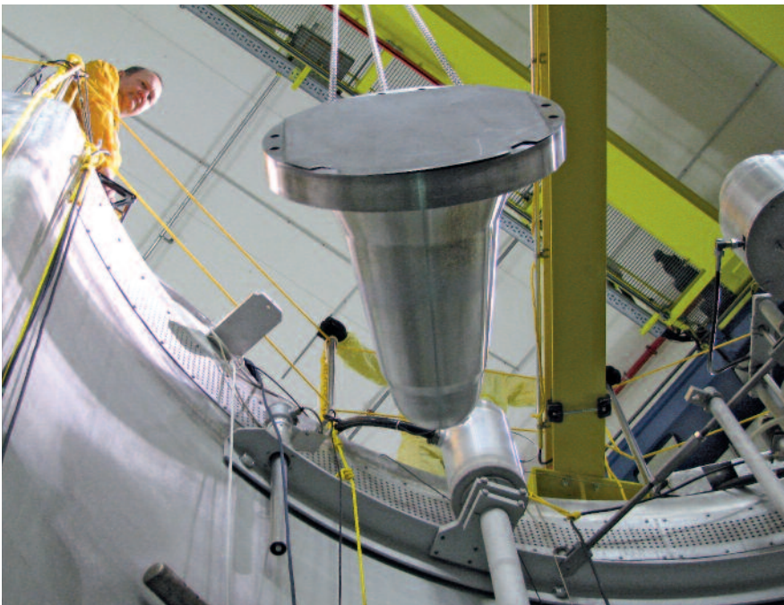
The conical beam tube is brought into position.
