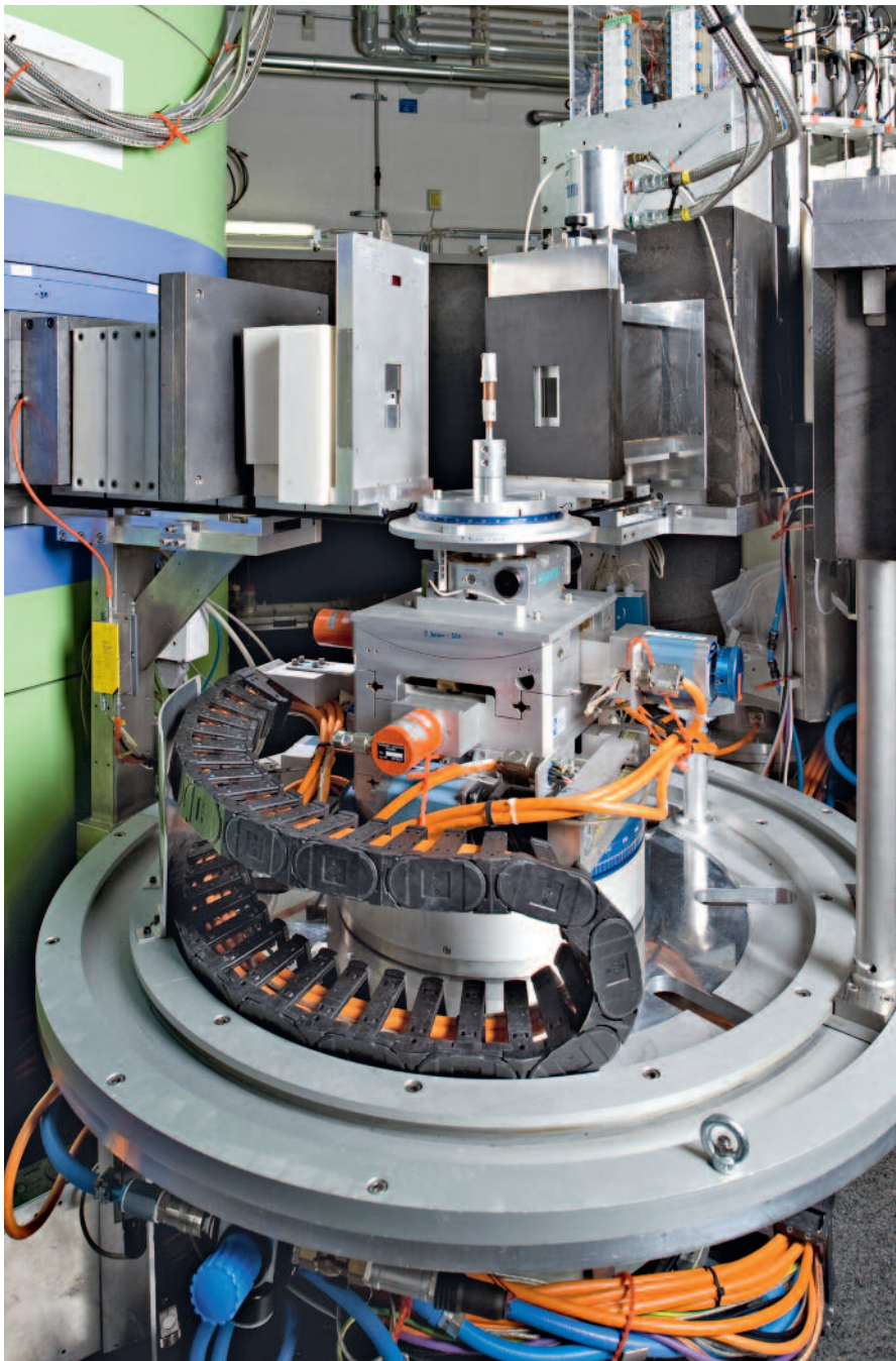
The cold neutron three-axis spectrometer PANDA operated by HZB at the Heinz-Meier-Leibnitz research neutron source (FRM II) in Garching near Munich was used for studying two iron-based superconductors.
