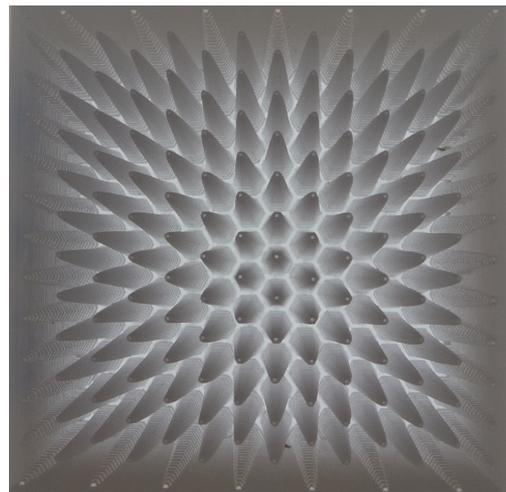
Figure 4: Close-up photo of the 3D printed ridge-filter modulator. The peaks are pointing downstream.
