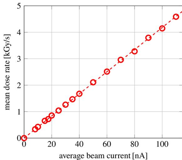
Figure 1: Measured mean dose rate against average beam current for a focused beam at full energy.
