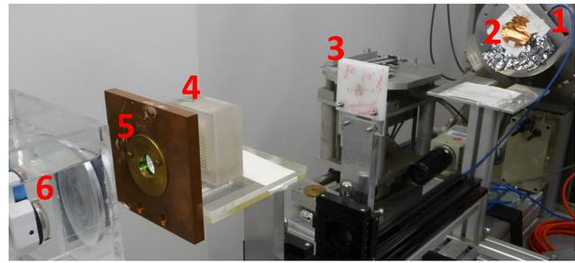
Figure 3: Beam nozzle with a dual-ring double scattering scheme (elements 2 and 3) and a static modulator (4). The beam travels from the vacuum window (1) to the dose chamber (6) through a collimating aperture (5).
